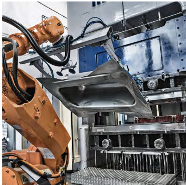
Today, the blanks are drawn and shaped from a single piece using our deep drawing press
