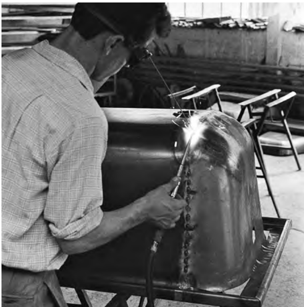
The bathtub blanks were previously welded together from three parts (1948)
